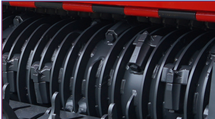
"Patented" rotor, hammers w/tungsten carbide tips
